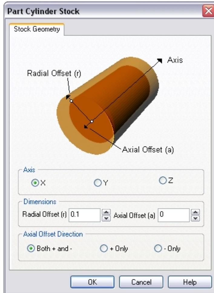
The user can define the cylinder by simply selecting the axis of the cylinder (either X, Y or Z) and defining the radial and the axial offset distances. The bounding cylinder will be calculated and these offset values will be used to expand the cylinder in both the radial and axial direction.
