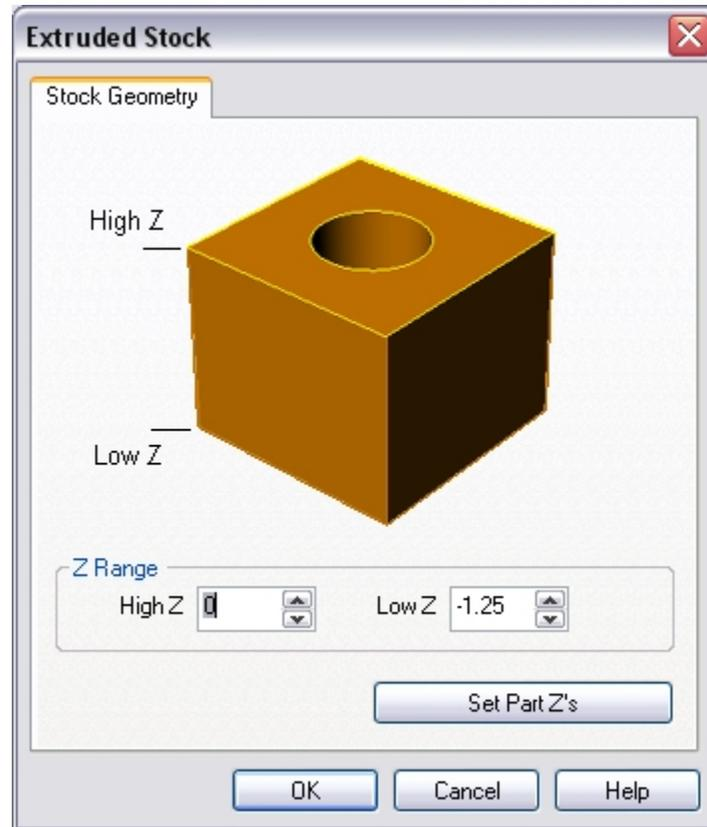
When the user clicks on the OK button, a stock model based on the selected regions and user definitions will be created. The user can switch to the Simulate tab of the browser window to display the stock model that was created.
