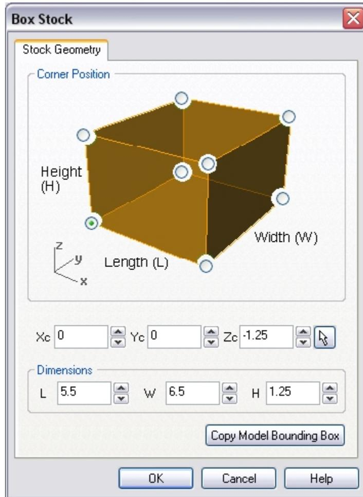
The user can define the box by simply typing in the length; width and height of the box in the corresponding edit boxes of the dialog. The corner position (origin) of the box can also be repositioned by picking the desired coordinate or by specifying the coordinate values in the corresponding edit boxes in the dialog (Xc, Yc, Zc). When the user clicks on the OK button, a stock model based on the user definition will be created and displayed.
