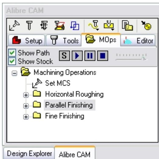
**Step 4: Simulate machining operations**
