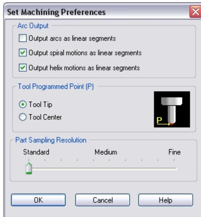
**Arc Output:** Some of the controllers do not have arc, spiral and helical output (for example G2, G3). For such type of controllers, the arcs that are generated in the Alibre CAM toolpath can be output as linear segments using this option.
