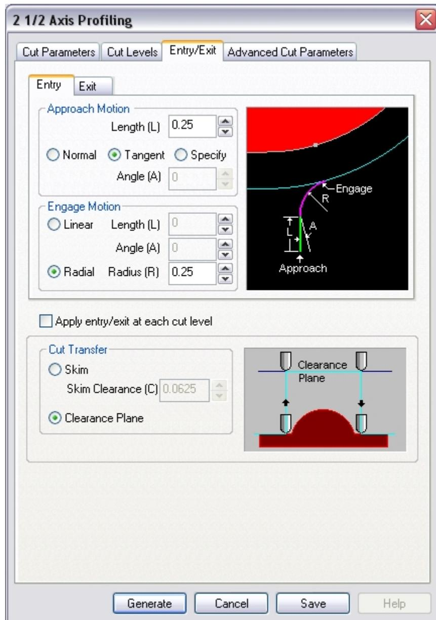
The Entry motion consists of Approach and Engage. The user can set different feeds for plunge, approach, engage, cut, retract and depart moves. The tool moves to the position above the approach point with a plunge feed, then uses the approach feed rate for the vertical approach motion and engage feed rate for the engage motion.
