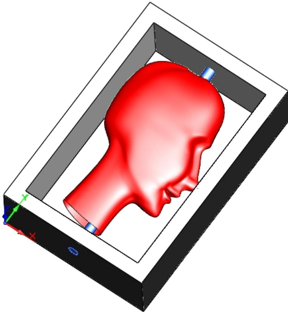
It should be noted that Alibre CAM allows for any user defined indexing angle and is not restricted to 180 degrees. This feature allows the user to machine multi-sided parts and not just two sided parts as the one shown above.
