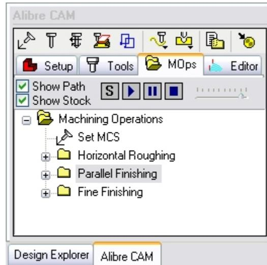
“MOPs” stands for Machining Operations. All toolpaths you create are listed here, in order of creation. Within each toolpath folder you can edit its various components, such as tool, regions, or cut parameters, by double-clicking the relevant icon. Right-clicking on a toolpath name provides several options, including simulation, generation, and post-processing.
