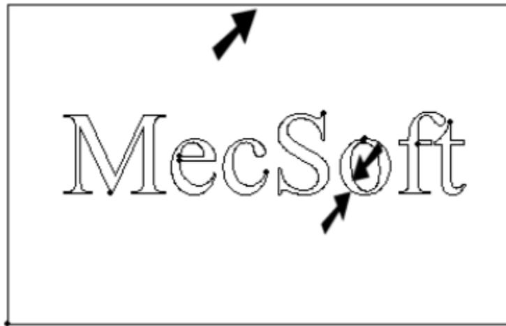
Note: The outer region should encompass the stock. You can easily create this type of region by selecting Bounding Region from the Curves category of the Geometry bar.
