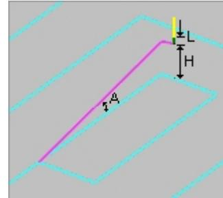
**Linear:** Here the cutter follows a linear ramp motion, ramping back and forth from a user specified height to the engage point. The length of this move, as well as the angle of this motion can be specified by the user.
