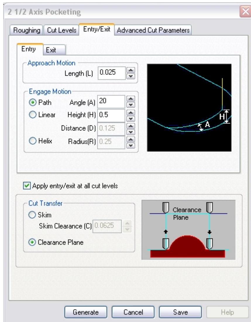
The Entry motion consists of Approach and Engage. The user can set different feeds for plunge, approach, engage, cut, retract and depart moves. The tool moves to the position above the approach point with a plunge feed, then uses the approach feed rate for the vertical approach motion and engage feed rate for the engage motion.
