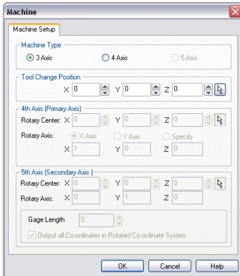
**Machine Type:** Allows the user to specify the machine type.
