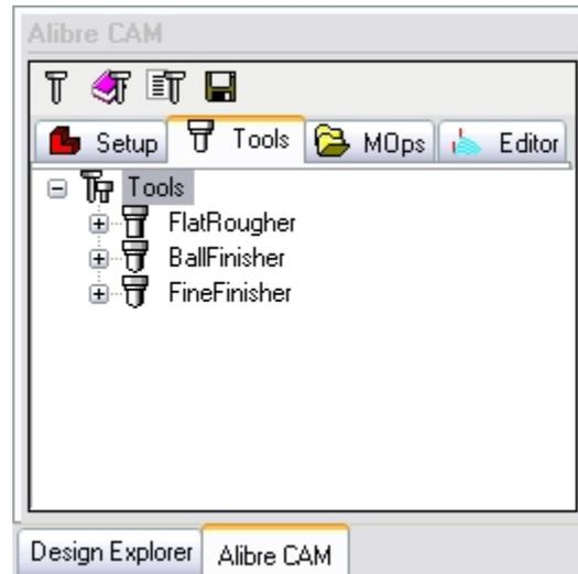
This tab lists all tools currently defined in the file. If you have created machining operations, the toolpath will appear in the **Tools** tab underneath the tool it uses. You can rename and delete tools, but you cannot delete a tool that is used in a toolpath. Double-click a tool icon to edit its parameters.
