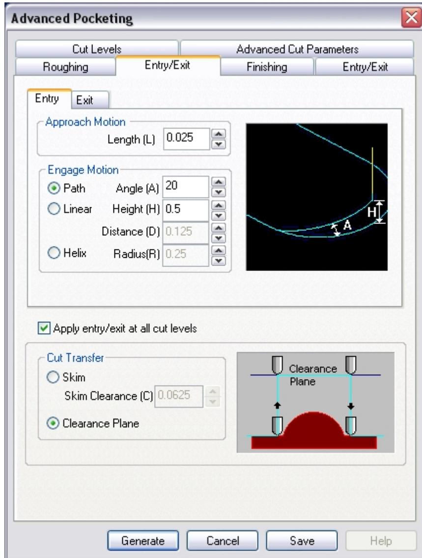
The Entry motion consists of Approach and Engage. The user can set different feeds for plunge, approach, engage, cut, retract and depart moves. The tool moves to the position above the approach point with a plunge feed, then uses the approach feed rate for the vertical approach motion and engage feed rate for the engage motion.
