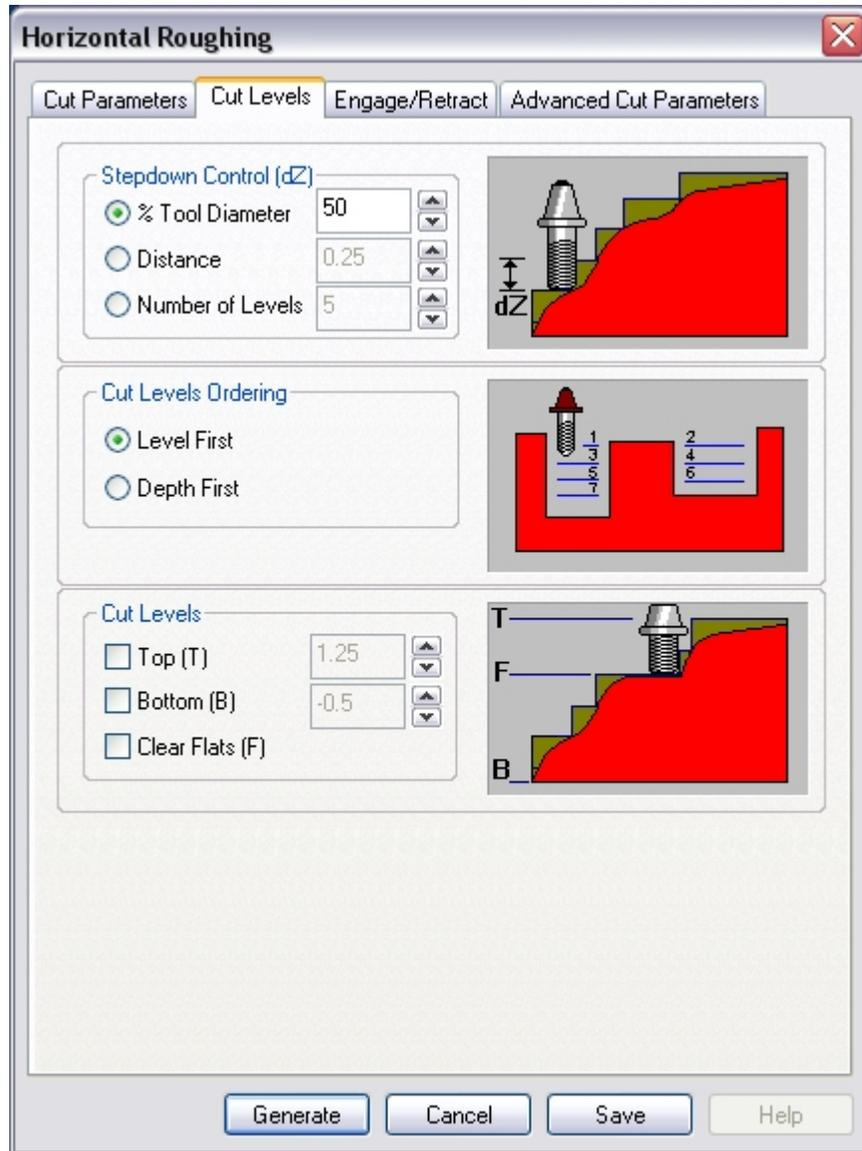
The Step-down Control section allows the user to define the spacing between the horizontal cut levels for the roughing operation. The spacing can be specified either as a percentage of tool diameter, a specific distance or as the total number of levels desired.
