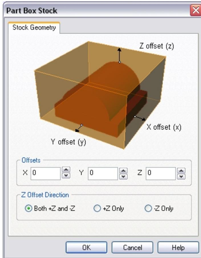
The system calculates the bounding box of the part model as the XYZ extents of geometry of the part model. The user can then define offsets in any of the three coordinate directions to apply to the computed bounding box. The system will expand the bounding box by the offset amount in each of the coordinate directions. When the user clicks on the OK button, a stock model based on the user definition will be created and displayed.
