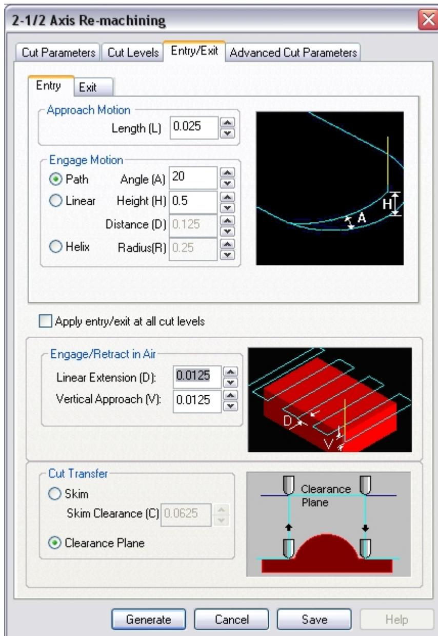
The Entry motion consists of Approach and Engage. The user can set different feeds for plunge, approach, engage, cut, retract and depart moves. The tool moves to the position above the
