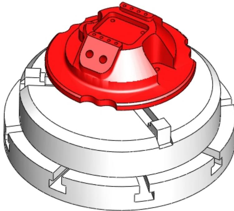
It should be noted that Alibre CAM allows for any user defined indexing angle and is not restricted to 180 degrees. This feature allows the user to machine multi-sided parts.
