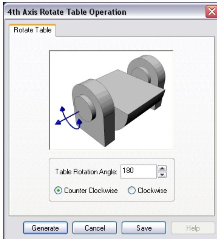
**Table Rotation Angle** - Specify the rotation angle value in degrees. When the user selects the Generate button, a Rotate Table machining operation will be created and displayed in the browser. When this operation is post processed and sent to the machine tool, a table rotation of the specified angle will be performed.
