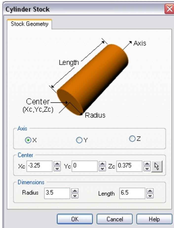
The user can define the cylinder by simply selecting the axis of the cylinder (either X Y or Z), specifying the center coordinates by typing in the values or graphically picking the center and then by specifying the radius and the length of the cylinder.
