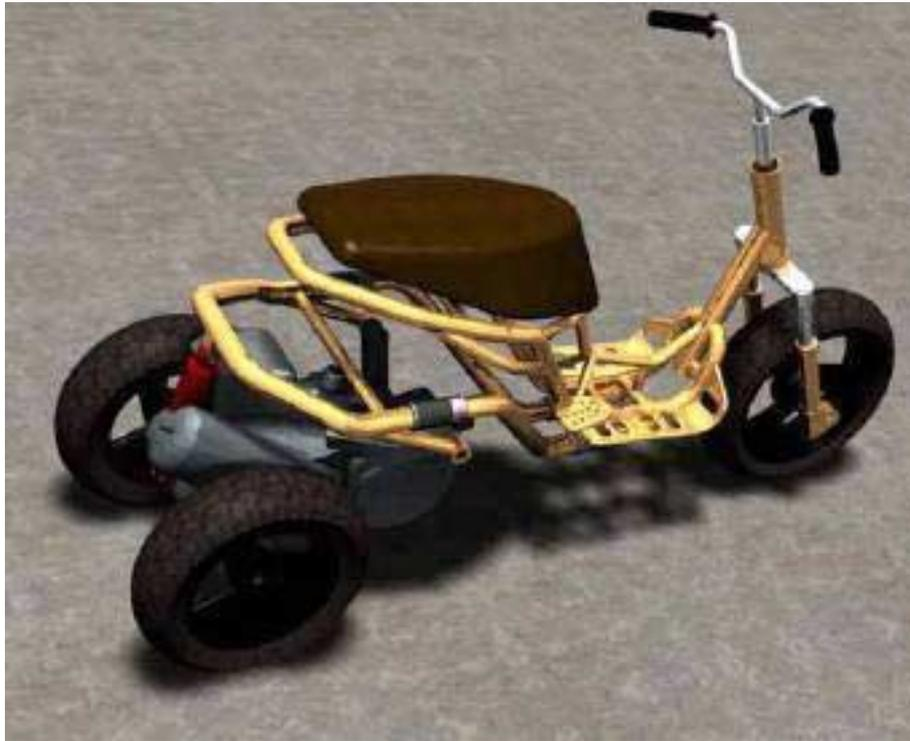
**Figure 16 – Tricycle virtual model screenshot made with visualNastran Motion**
