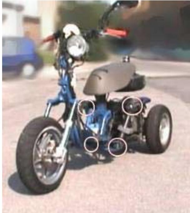
**Figure 25 - Prototype built at the department. Revolute joints highlighted**
