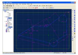
Sketch Constraints. The intelligent sketcher automatically detects and infers relationships between sketch entities and construction geometry, capturing sketch constraints on the fly. Sketch constraints, which can also be applied manually, include:
