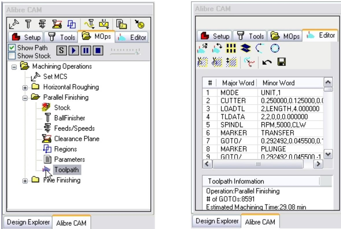
The dialog shows the Edits on the top with a list box that lists the tool motions that can be edited. Below this list box there is another list box that displays the operation name, the number of toolpath points as well as the estimated machining time. The user can remove individual tool motions from the tool path by selecting the desired lines.
