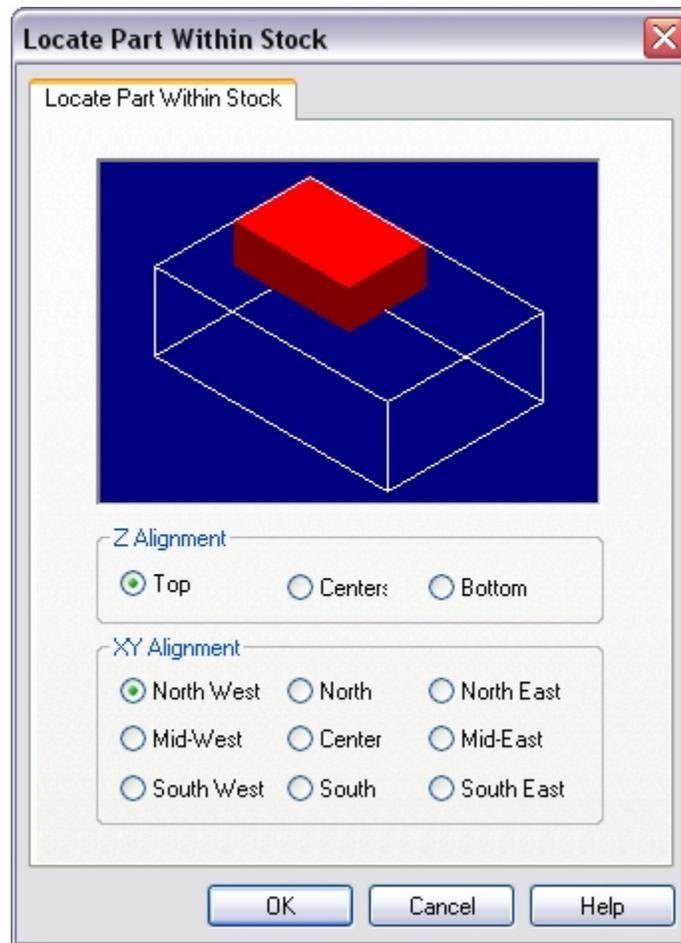
Z alignment of the stock can be set to the Top / Center / Bottom of the part geometry and the XY alignment can be set to one of the configurations shown in the dialog box above.
