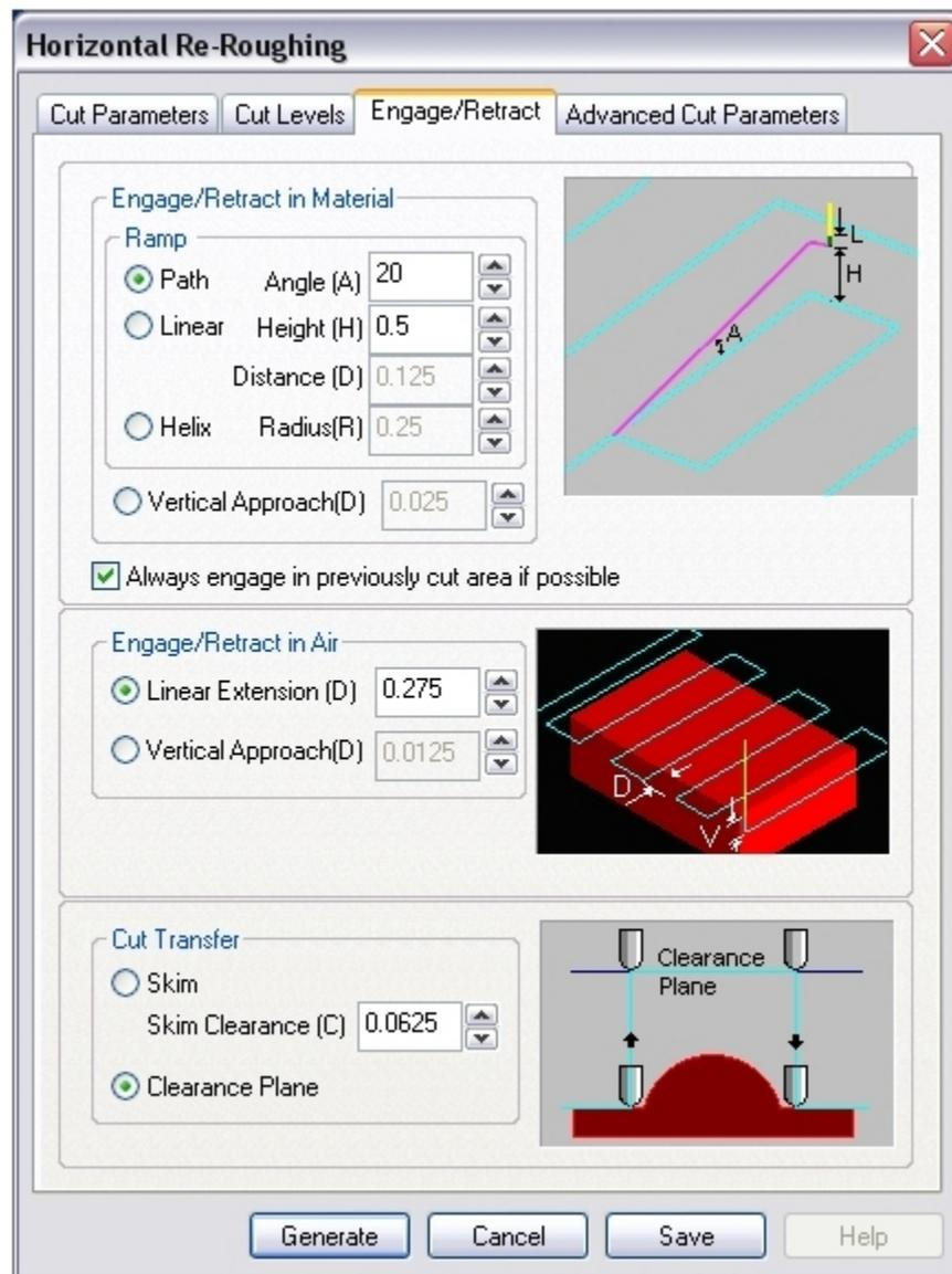
The Engage in Material section allows the user to define how the cutter would engage into material when forced into such a situation. This can happen when machining a cavity or pocket. The user
