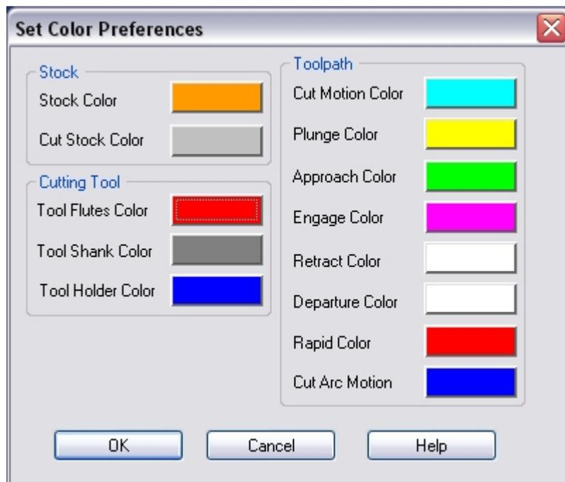
**Cutting Tool Colors** - Set the tool's flute (cutting portion) and the shank's (non-cutting portion) color in this section.
