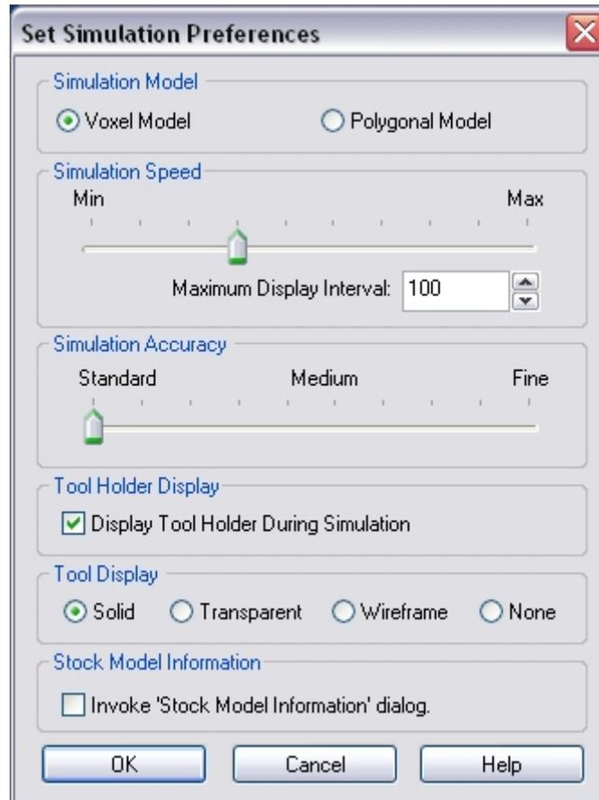
**Simulation Model:** In Alibre CAM the user can choose between two simulation models. One is called the Voxel Model and the other the Polygonal Model.
