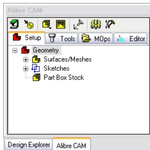
The Setup manager displays the three types of geometry that can be created and manipulated in Alibre CAM: **Surfaces/Meshes**, **Sketches** and **Stock**
