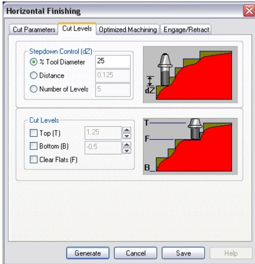
The Stepdown Control section allows the user to define the spacing between the horizontal cut levels for the roughing operation. The spacing can be specified either as a percentage of tool diameter, a specific distance or as the total number of levels desired.
