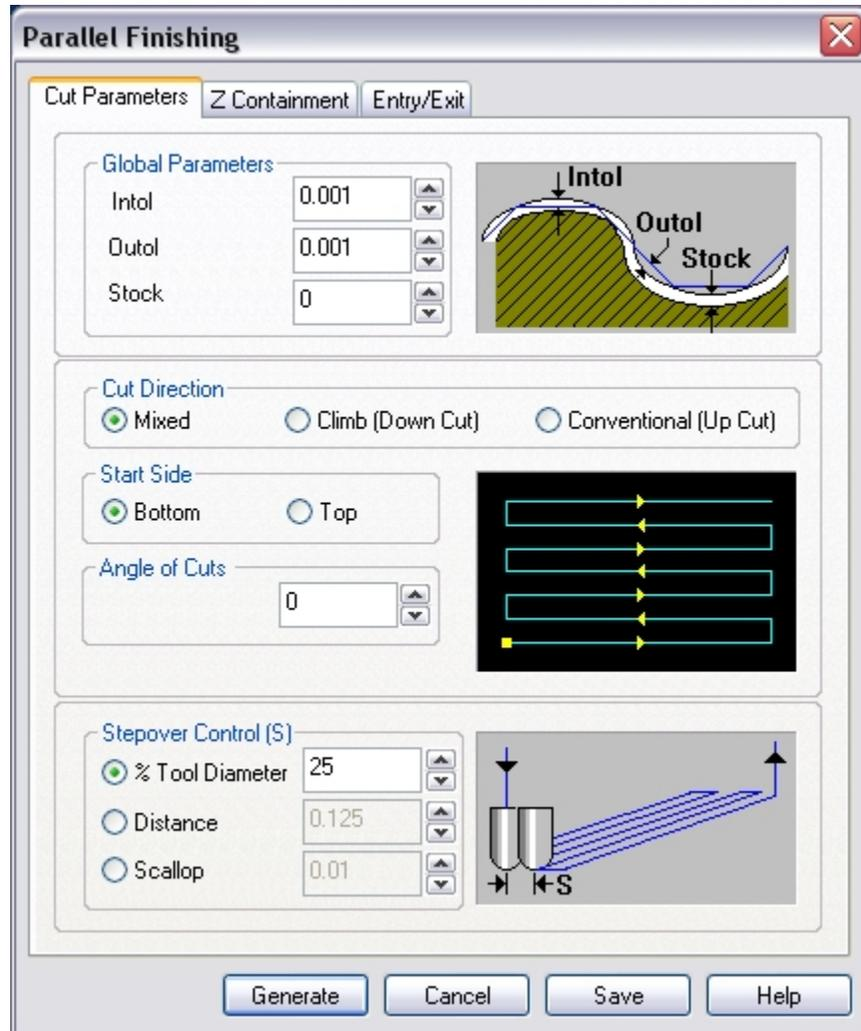
This dialog is a tabbed dialog with two tabs. Clicking on each of the tabs allows the user to set the different parameters. The following sections describe each of the tabs in more detail.
