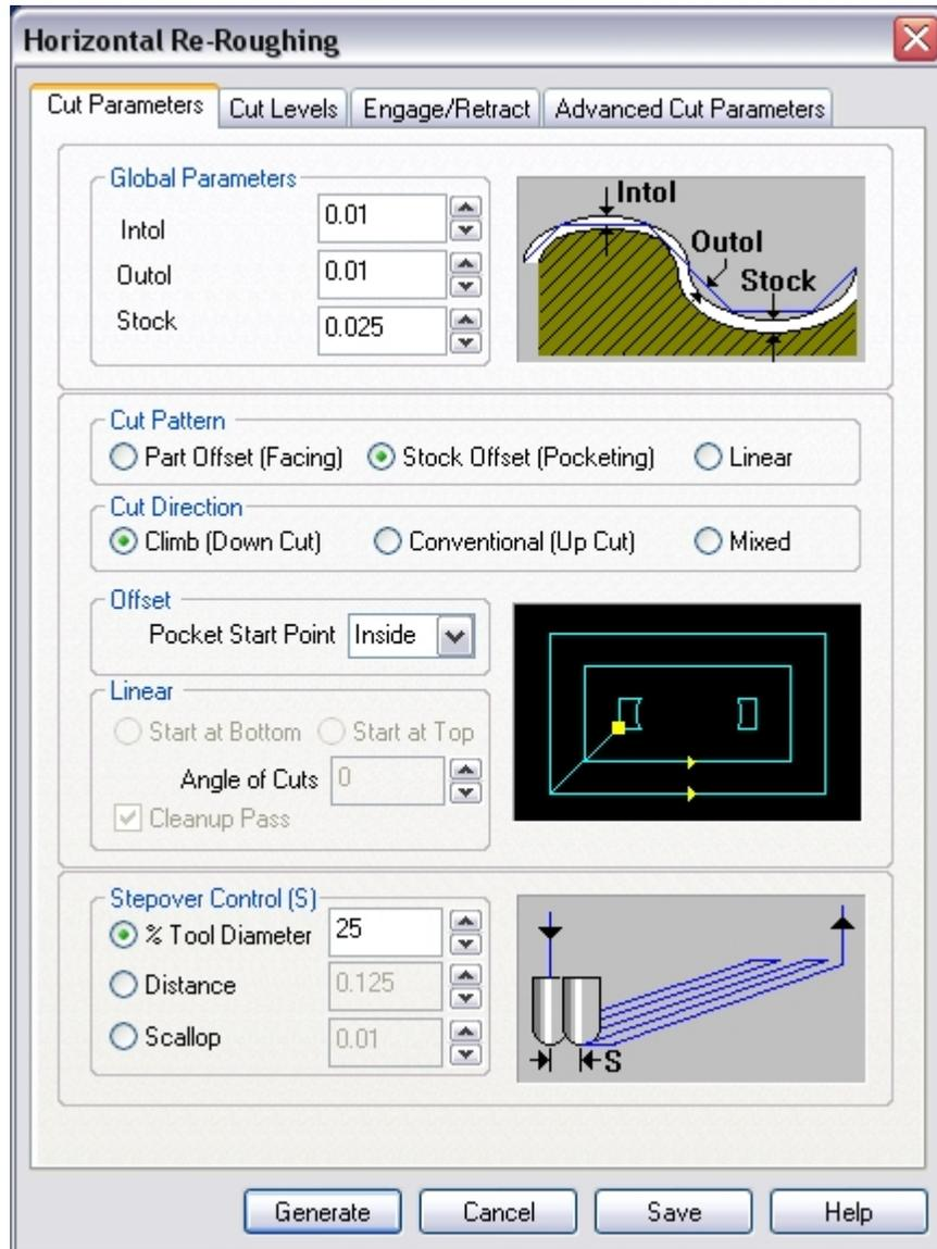
This dialog is a tabbed dialog with three tabs. Clicking on each of the tabs allows the user to set the different parameters. The following sections describe each of the tabs in more detail.
