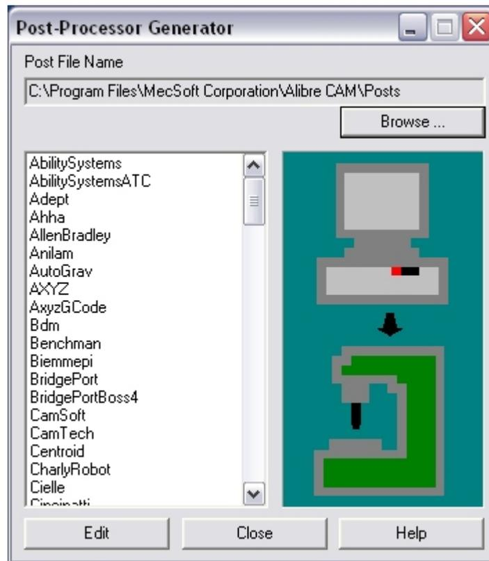
To create a new post-processor, define the parameters and click **Save As**. A new spm file will be created in the **Post** folder.
