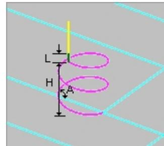
The Engage in Air section allows the user to define how the cutter would engage to start cutting when starting from outside of the part. This can happen when machining a core or performing a facing operation. In such cases the user has the option of specifying the cutter to start from the outside, a certain distance away from the cut start point. Or optionally a straight vertical engage can be specified.
