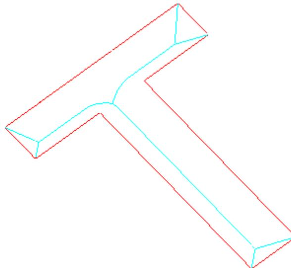
The unique feature of this type of toolpath is that the V-cutter creates a chiseled look at the corners by moving the cutter tangent to both converging sides of the corner.
