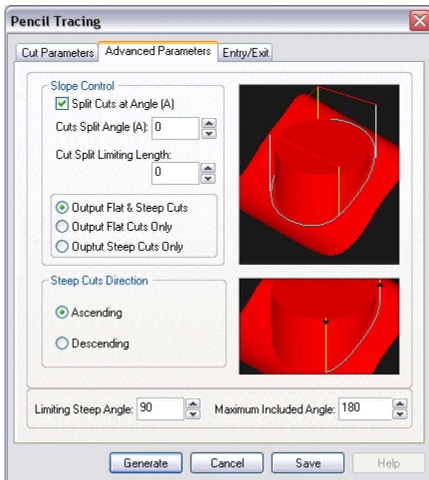
This section of the dialog is used to control the cuts based on the slope of the cuts.
