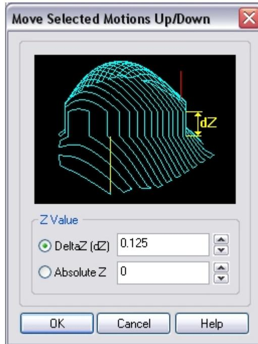
In the first case the toolpath selection is merely shifted up in Z by the delta amount. In the second case, the starting point of the selection is moved to the specified absolute Z coordinate. All other selections will be shifted up by the same relative amount as the first point of the toolpath point.
