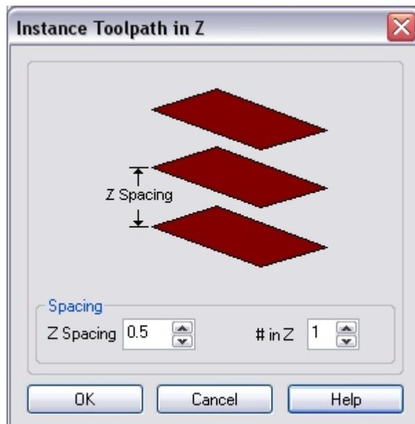
The user can specify the number of instances in Z as well as the spacing between the Z instances. The toolpath will be copied multiple times and the tool initial engage will start from the top-most instance and work its way to the bottom most instance. Negative values can be specified in the Z spacing. In this case the instances will proceed below the current location of the toolpath.
