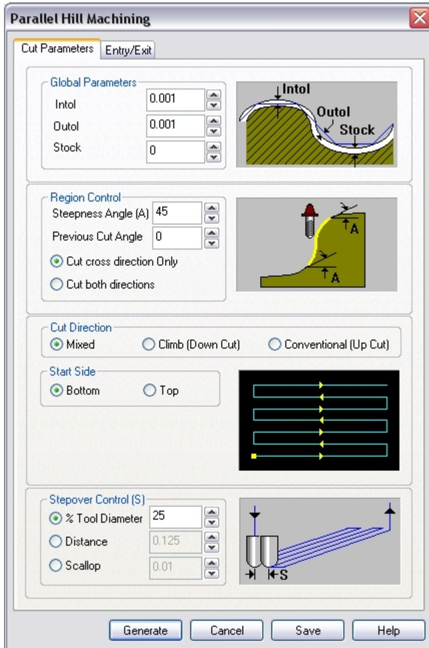
This dialog is a tabbed dialog with two tabs. Clicking on each of the tabs allows the user to set the different parameters. The following sections describe each of the tabs in more detail.
