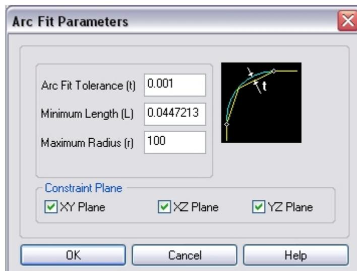
The user specifies an arc fitting tolerance, a limiting arc length as well as the smallest radius of the arc allowed. The arc motions can further be restricted to be created in any or all of the principal planes.
