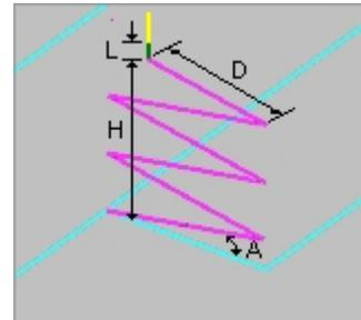
**Helix:** Here the cutter follows a helix as it descends from a user-defined height to the first cut point. The angle of the helix as well as the radius of the helix can be specified by the user.
