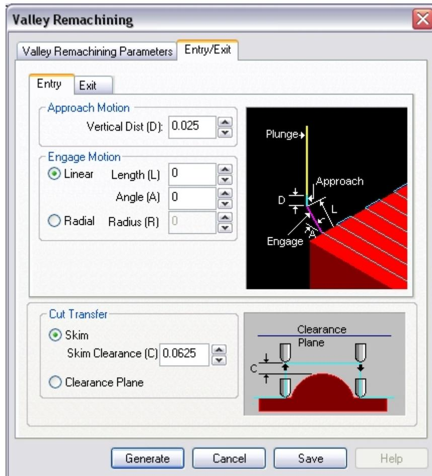
The user can also control the transfer motions during cutting. When the cutter has finished cutting in one region and needs to transfer to another region to begin cutting, it can either be instructed to
