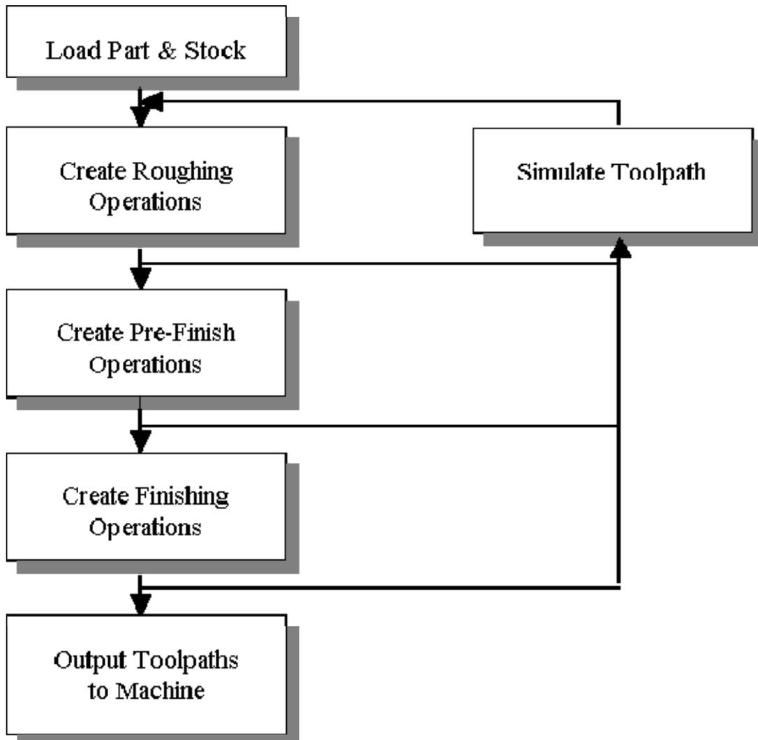
Part geometry is loaded into Alibre CAM via the various data interfaces provided in Alibre. A stock model representing the raw stock from which the part needs to be manufactured can then be created using the various tools provided in Alibre CAM.
