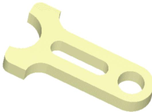
Using this class of machining, you can machine parts that are defined only by 2D curves. 3D part geometry can be present, though it is not necessary.
