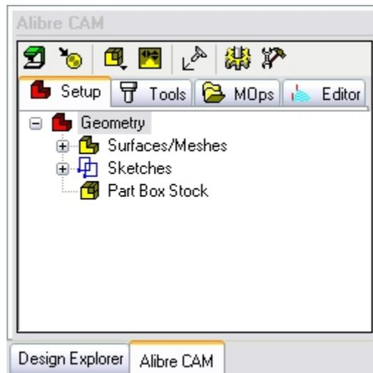
Users can switch between the Design Explorer and Alibre CAM by switching tabs at the bottom of the Alibre CAM browser.
