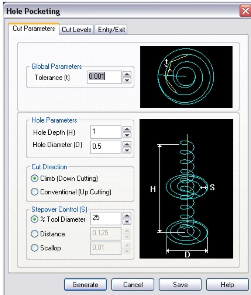
This dialog is a tabbed dialog with three tabs. Clicking on each of the tabs allows the user to set the different parameters. The following sections describe each of the tabs in more detail.
