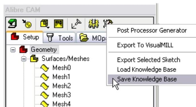
This will allow the user to save this entire sequence of operations and all of the associated operation parameters in an external VKB file.
