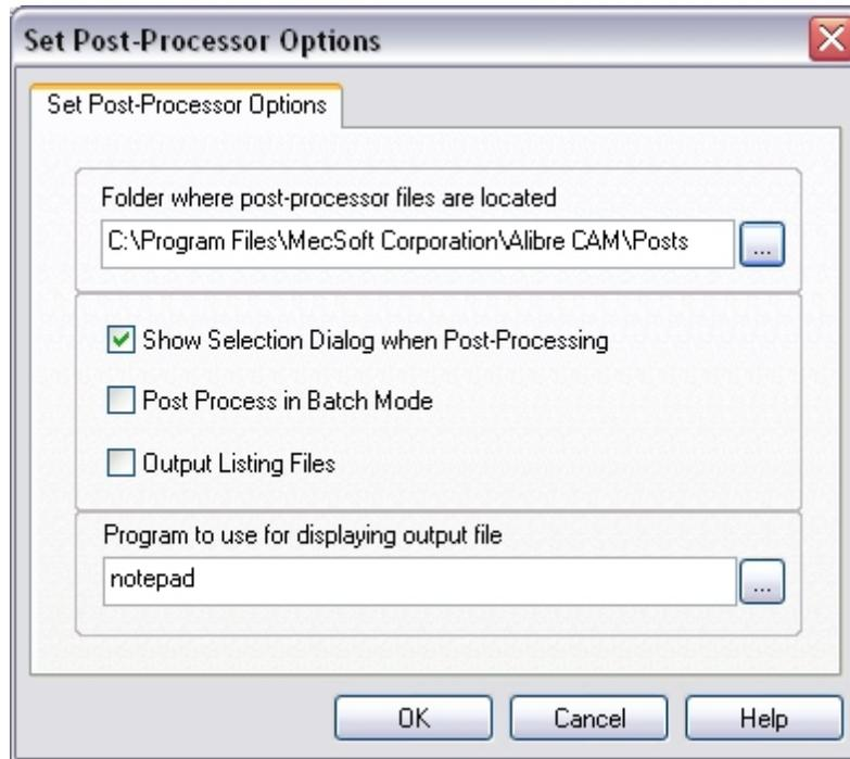
Alibre CAM by default performs interactive post-processing. That is, when the user selects a toolpath for post-processing, Alibre CAM launches the post-processor and waits for the post-processor to complete. The user can specify Alibre CAM not to wait for the completion of the post-processor. This is done by checking on the Batch Mode check box in this dialog. The user also has the option to output the list files and display the selection dialog for each post processing operation.
