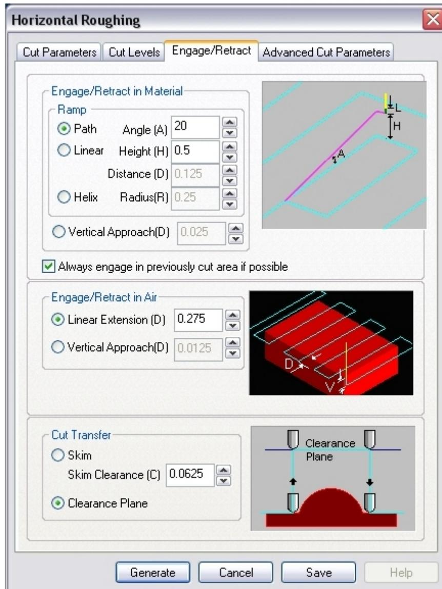
The Engage in Material section allows the user to define how the cutter would engage into material when forced into such a situation. This can happen when machining a cavity or pocket. The user has the option of Ramping the cutter or engaging vertically down. The ramp engage motion will typically be used when machining with a flat or corner-radius end mills.
