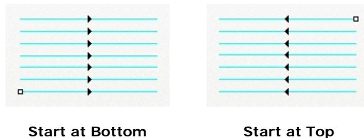
The Stepover Control section allows the user to define the spacing between the cuts. The spacing can be specified either as a percentage of tool diameter, a specific distance or as the scallop height.
