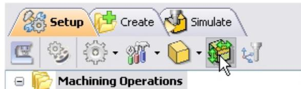
2. Set Z alignment to **Center** and XY alignment to **Center**. (This would align the stock to the top of the part in Z and center in XY)
