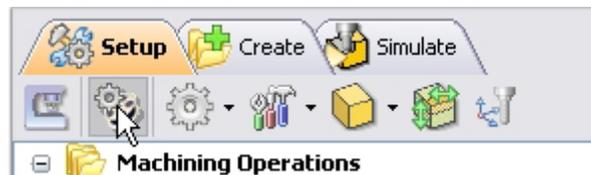
5. Set the current post processor that is on your controller. We will select Haas as the post processor for this exercise. Set the posted file extension type to .nc
