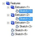
Note: You can also select the sketch from Alibre Design View. When select containment region is selected, Alibre CAM turns on Sketch selection filter to allow the user to select sketches. Hold the Shift key down to select multiple sketches.
