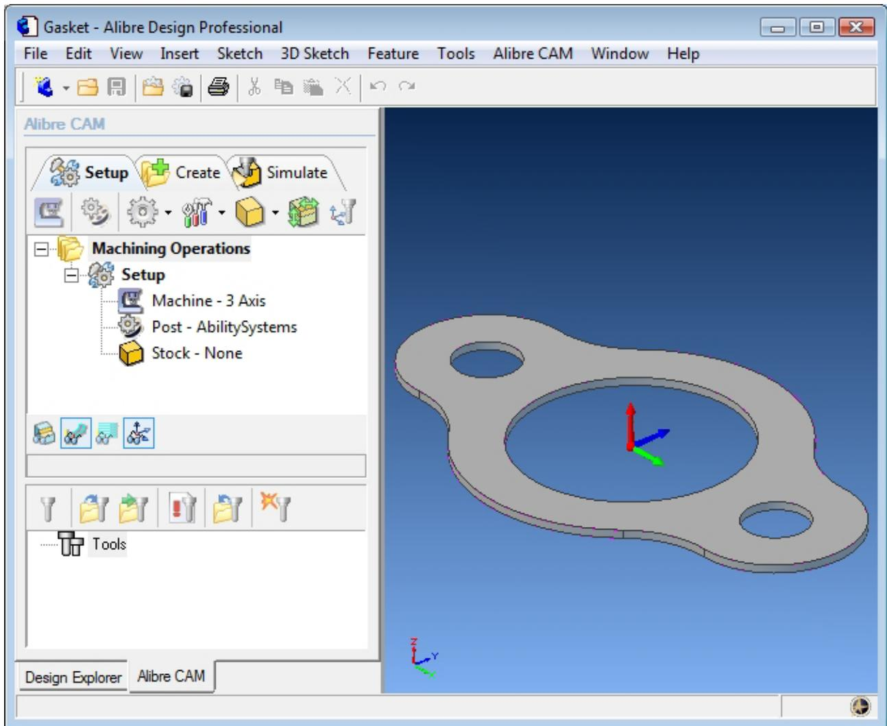
The Alibre CAM browser (MOPs and Cutting Tools) is now loaded and is docked over the Design Explorer. You can toggle between the MOPs browser and the Design Explorer from the tabs at the bottom of the window. It can be hidden by un-checking Browser on the Alibre CAM menu bar. To re-display the hidden Browser window, you can re-check **Browser** from the Alibre CAM menu entry. You can also resize it by dragging one of its sides.
