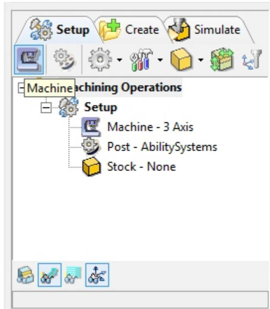
2. Set the Machine Type to 3 Axis. Click Ok Close the Setup Machine Dialog.
