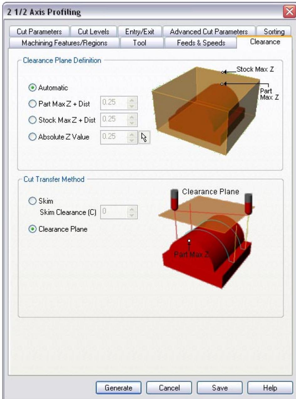
11. Set the Clearance Plane Definition to Automatic and Cut Transfer Method to Clearance Plane.
