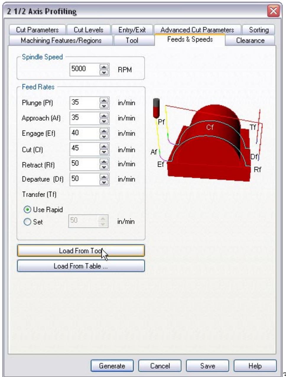
9. Select Load From Tool. Alibre CAM will now get the feeds and speeds information that was set when the tool was defined.
