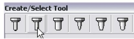
2. Set the tool name as **FlatMill-0.5**, Tool Diameter = **0.5**, Under the Properties tab set Tool Number = **1**.
