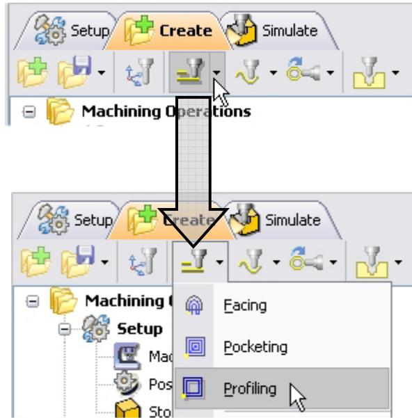
This brings up the 2 ½ Axis Profiling Operations dialog. We will go over the steps for creating the profile operations for the inner features of the Gasket.
