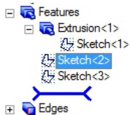
Note: You can also select the sketch from Alibre Design View. When select containment region is selected, Alibre CAM turns on Sketch selection filter to allow the user to select sketches. Hold the Shift key down to select multiple sketches.
