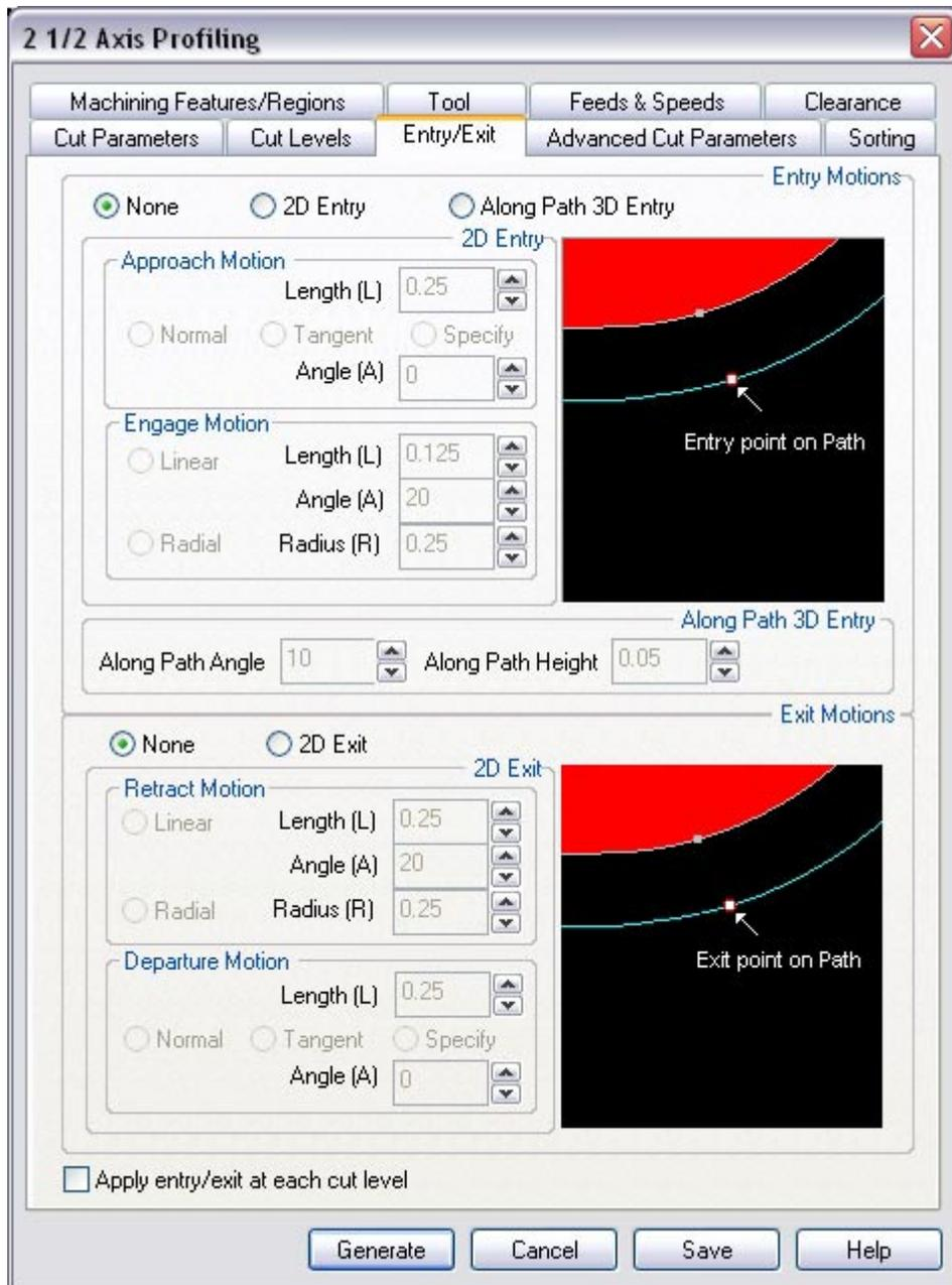
16. Click Generate. The 2½ Axis Profile toolpath is now generated and the Operation is listed under the Alibre CAM-MOPs browser.
