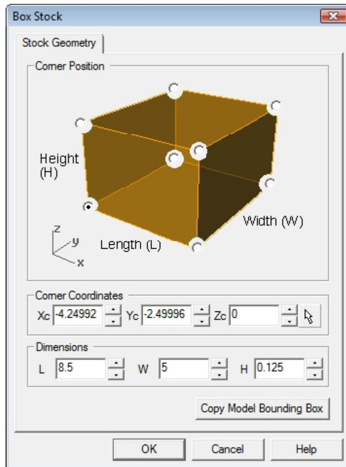
7. The stock geometry is now created, and a semi-transparent stock box is displayed on top of the part geometry.
