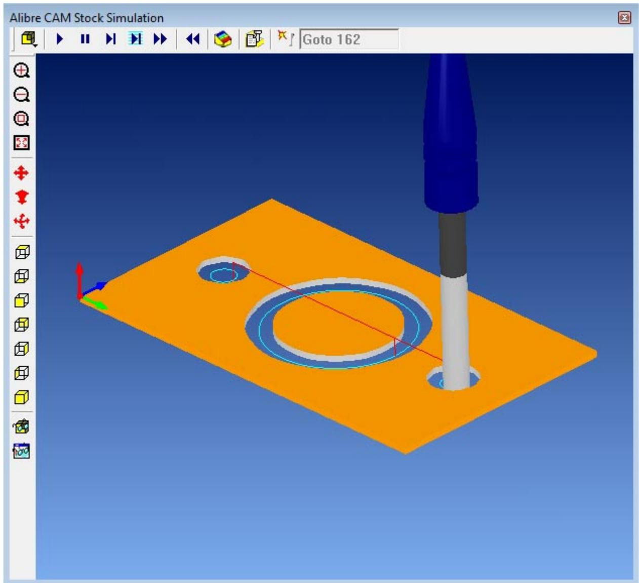
Note: You can pause/stop, step, and skip the simulation using the controls available on the simulation window. To control the simulation speed, select Simulation Settings from the Stock Simulation window.
