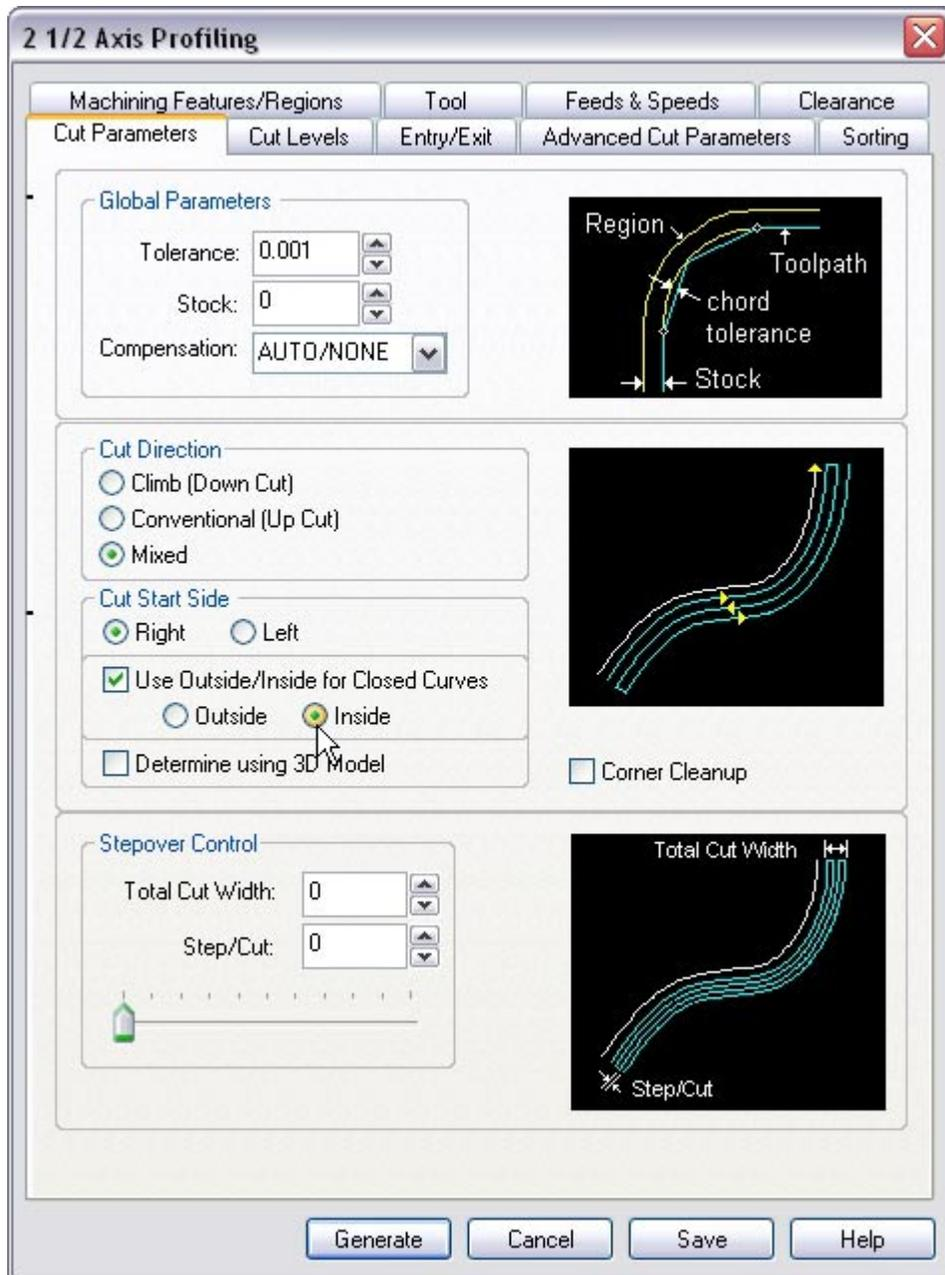
13. Set the Stock = 0 and under cut start Side check Use Outside/Inside for Closed Curves and select Inside. Alternatively you can also use Determine using 3D model.
