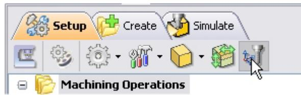
2. Switch to SetMCS Origin tab and choose **Set to Stock Box**, the Zero Face to **Highest Z**, and Zero Position to **South West** corner. This sets the machine home to the top of the stock material and the southwest corner of the part geometry.
