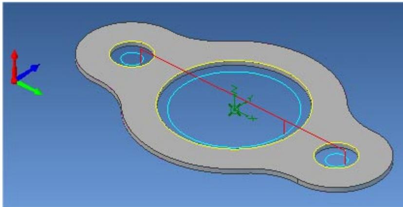
1. Right mouse click on the 2.5 axis Profile operation and rename the operation to Inner Profile.
