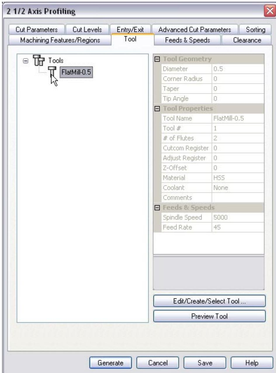
7. Select the FlatMill-0.5. The 0.5" Flat End mill is now selected as the active tool and the Tool parameters are displayed to the right of the Tools window.
