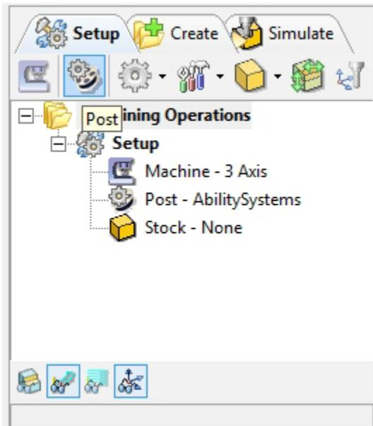
4. Set the current post processor that is on your controller. We will select Haas as the post processor for this exercise. Set the posted file extension type to .nc
