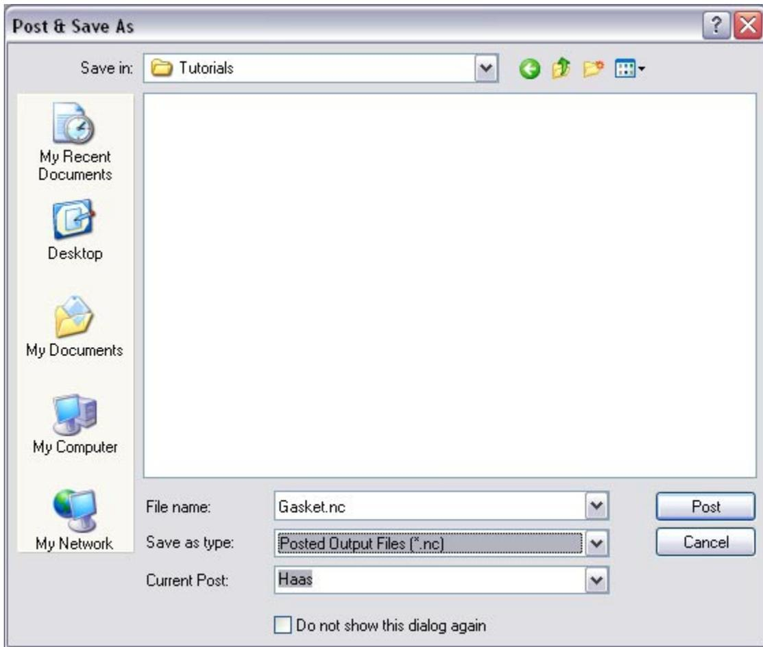
*The post by default is set to Haas as specified under the Post processor setup. You can change the post processor by selecting a different one from the drop down menu in the list. The posted g code by default will be saved to the folder where the part file is located.*
