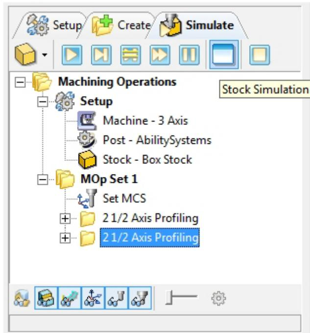
2. Click Simulate from the Stock Simulation window to run simulation.
