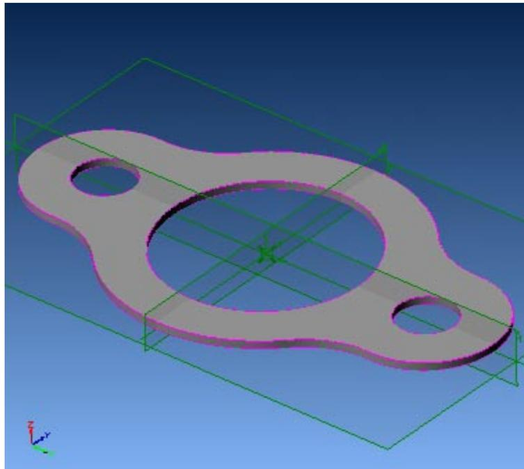
**Note:** You must work in shaded mode in order to be able to visualize toolpaths created in Alibre CAM. It is suggested for best visual performance with Alibre CAM to work with only one view port open and the view port operating in shaded mode.
