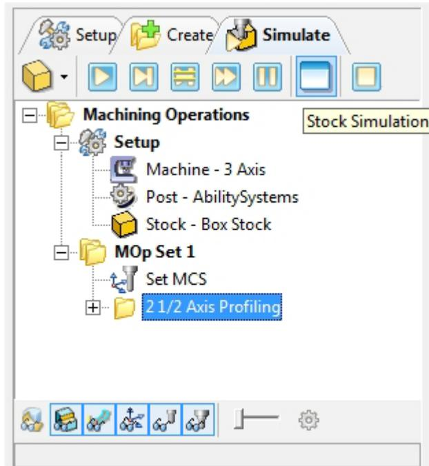
2. Click Simulate from the Stock Simulation window to run simulation.
